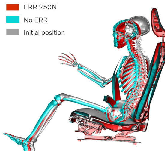
Fig. 6. Comparison of HBM positions at time of impact (800 ms) with respect to ERR function activation. The grey HBM shows the initial position at the start of the pre-crash phase (300 ms). The red HBM shows position at time of impact for the simulations with activated ERR function (simulations No. 2, 5, 7 and 9) and the turquoise HBM those without (simulations No. 3, 4, 6, 8 and 10).
