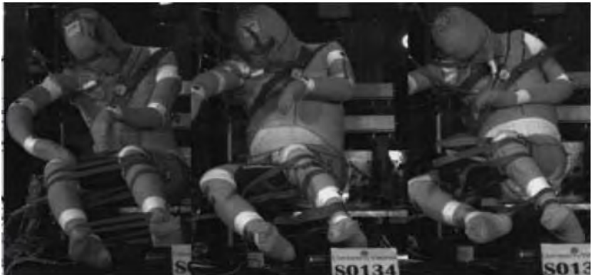
Fig. E 2. Test Configuration 3: SAFER HBM (left) and the three PMHS tests S0123, S0134, S0137 from [12] (right)
