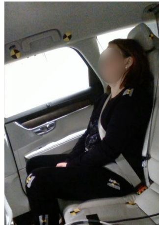
Fig. 7b. Participant 9 with shoulders in contact with the seat back during the stationary scenario, viewed from the side.
