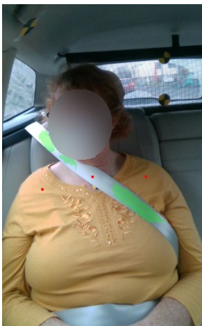
Fig. 9a. Participant 10 with the belt positioned close to the neck and armpit.
