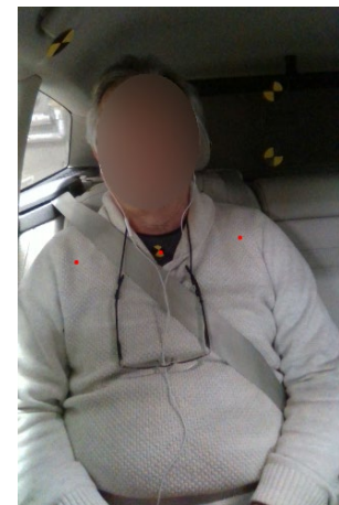
Fig. 8d. Participant 8 has the belt close to the neck during the stationary scenario.
