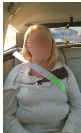
Fig. 9c. Participant 3 with the belt positioned close to the neck and armpit during the driven scenario.
