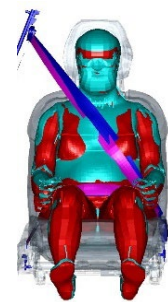
Fig. B.7. The initial shoulder-belt fit is compared between a female (red/magenta) and male (cyan/blue) occupant, with a stature of 1617 mm and BMI of 28 kg/m 2 . The belt is 19 mm more lateral relative to the clavicle for the female occupant.
