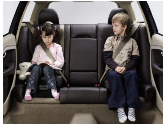
Figure 2b. Two stage integrated booster; high position (left) and low position (right)
