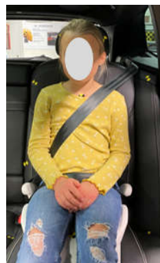
Figure 6b. 'Tall girl' restrained on the booster cushion concept in a vehicle rear seat; shoulder belt positioned over the guide.
