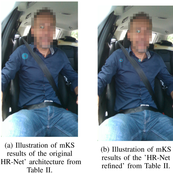
FIGURE 10. Comparison of predictions of original and refined HR-Net. The key point upper sternum is not present in the original network (Figure 10(a)) and the shoulder key point is not located as defined in Section II-B.
