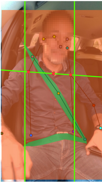
FIGURE 2. Example of one image in dataset X, annotated with COCO Annotator [19]; it supports bounding boxes, key points and polygons.
