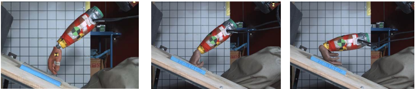
Fig. 2. Example of trajectory with hand in initial 30^\circ flexion orientation. Left: the fingers' first contact, mid: bottoming-out of the fingers, right: flexion with a bending moment of the wrist.
