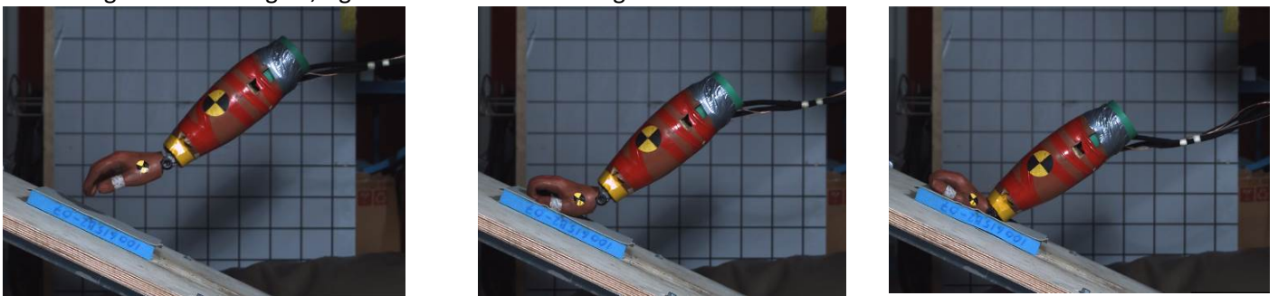
Fig. 3. Example of trajectory with hand in initial 35^\circ extension orientation. Left: the fingers' first contact, mid: extension of hand, start of wrist moment, right: forearm bottoming out.
