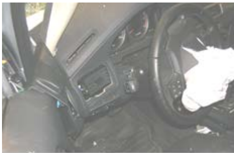
Fig. 4a. Photo of the left hand's impact area from the real world crashed car.
