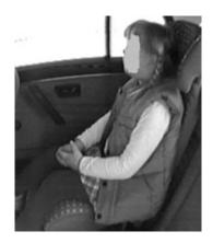
Figure 3b. The most common sagital sitting posture using the booster seat with the small head side supports in the study by Andersson et al. 2010.
