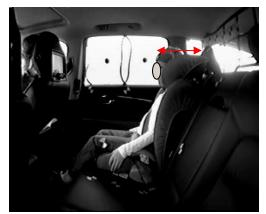
Figure 2b. Child 6 yo – 123 cm in rear seat of Volvo XC70 using booster seat with backrest.
