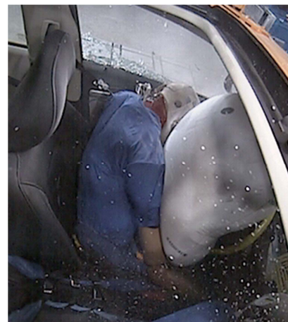
Figure 14. Interior view on occupant maximum forward displacement in car-to-barrier test set-up.
