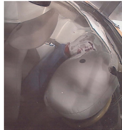
Figure 13. Interior view on occupant maximum forward displacement in car-to-car test set-up.
