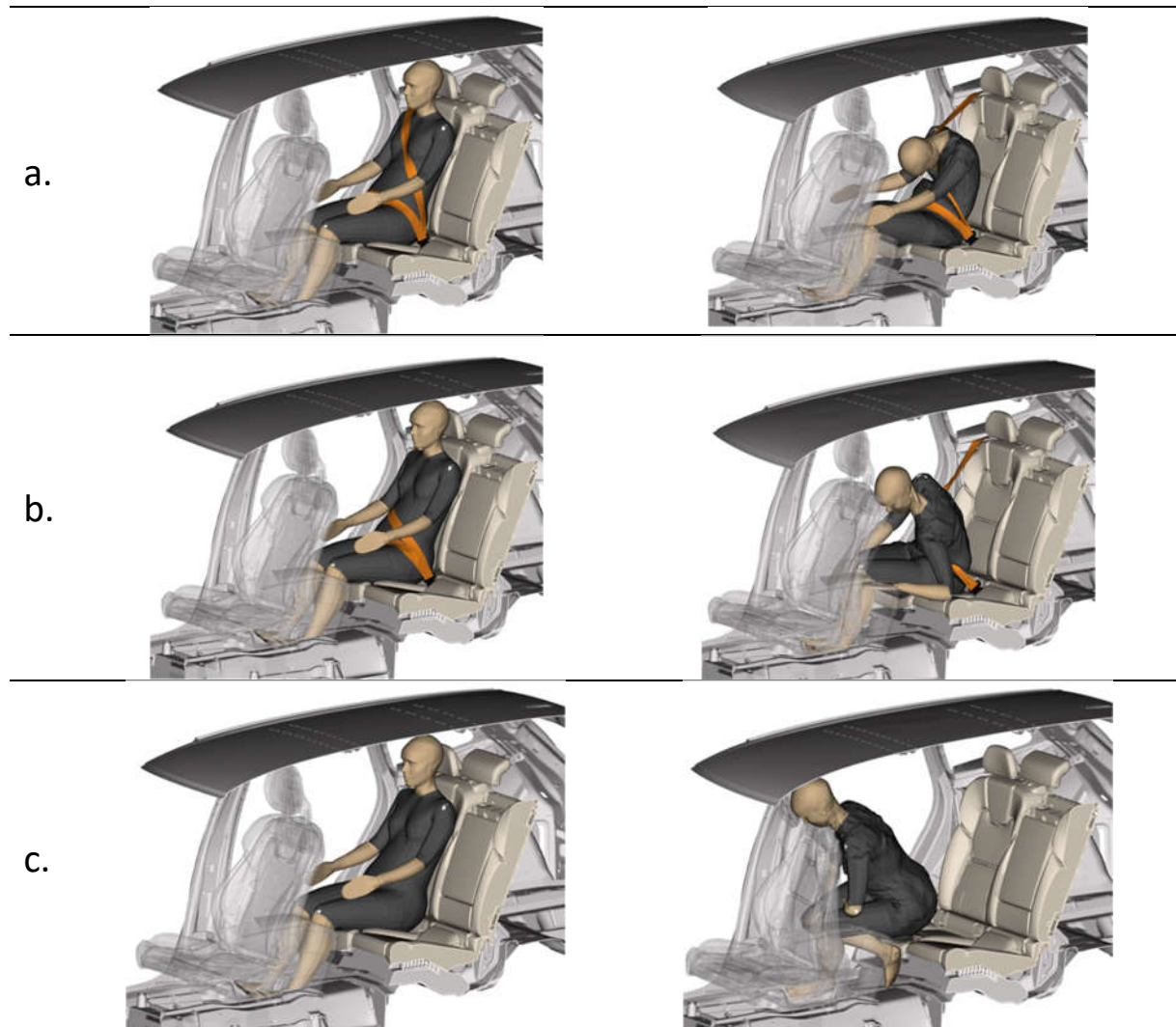
Figure 12. Crash simulations comparing occupant trajectories for a) correctly restrained, b) incorrectly restrained – belt under the arm, and c) unrestrained, with a rear-seated mid-sized female human body model, ViVA (Östh et al. 2017); Initial position (left) and most forward position (right).
