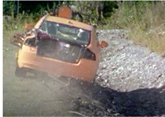
Figure A1b. Road departure test programmed into the robot rig.
