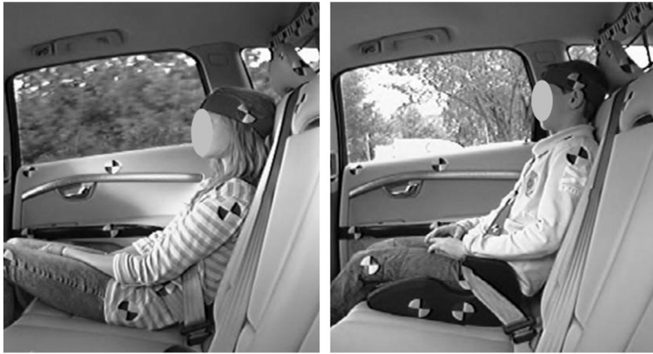
Fig. 7. Examples of slouch in [35] for a child seated directly on the rear seat (left) and a child of the same age seated on a belt positioning booster cushion (right).
