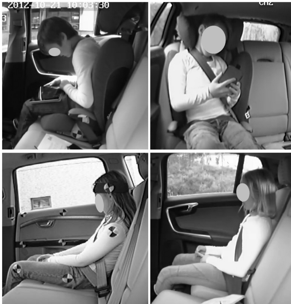
Fig. 6. Examples of voluntary seated postures in [31,35], from top left to bottom right: forward leaning posture when the child is playing with a smart phone; rotation of the upper torso to play with a smart phone when seated in a highback booster seat; slouching to comfortably accommodate bent knees when seated directly on the rear seat; child seated on an integrated booster.
