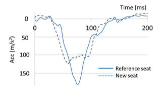
Figure 6. Pelvis vertical acceleration comparing new seat and reference seat using the virtual loading rig test method (Jakobsson et al. 2015).
