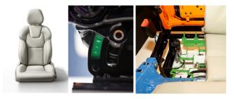
Figure 5. Overview of seat design including side bolsters (left). Close-up views of energy absorption functionality; side view of deformation element (middle), top view of seat cushion including springs (right).
