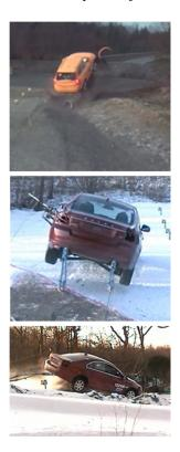
Figure 1. The complete vehicle Run off road crash test methods; Ditch (top), Airborne (middle) and Rough Terrain (bottom).
