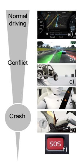
Figure 4. Holistic approach including countermeasures; Driver support system exemplified by a) Driver Alert Control with Rest Stop Guidance and b) Lane Keeping Aid, occupant protection systems exemplified by c) run off road detection, d) electrical reversible safety belt pre-tensioning and e) energy absorbing functionality in seat, and f) post-crash measure such as eCall activation.
