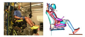
Figure 3. Rig test methods for vertical occupant loading; physical test setup (left) and virtual test setup (right).
