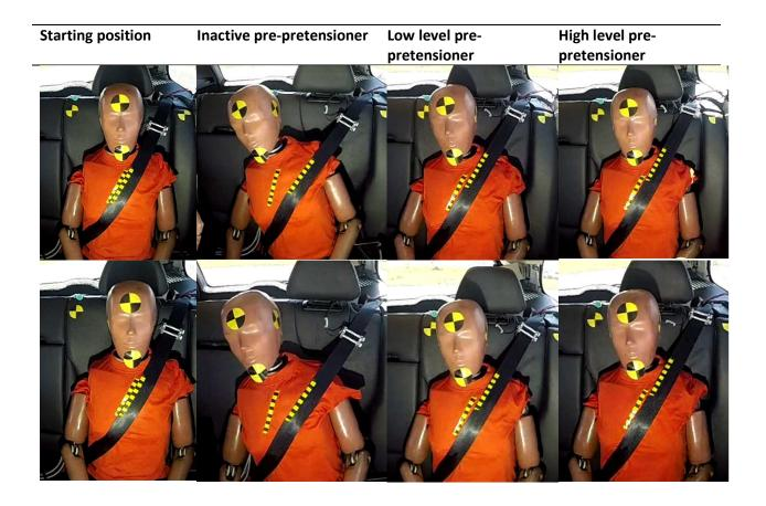
Figure 3 The left column shows the starting positions of the HIII5<sup>th</sup>, the next three columns shows the maximum lateral inboard motion restrained without pre-pretensioner activation (second column), pre-pretensioner low level (third column) and pre-pretensioner high level (fourth column). The first row shows the first sequences of tests and the second row shows the repeated tests.
