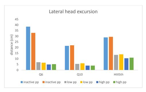
Figure 4 The lateral head excursion of the three ATDs, restrained without activation of pre-pretensioner (no pp), low level of pre-pretensioner force (low pp) and high level of pre-pretensioner force (high pp).
