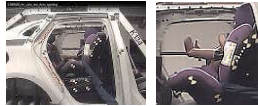
Figure 12b. Rearward facing seat, initial position (left) and maximum forward excursion (right). (Jakobsson et al., 2013)
