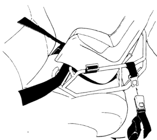
Fig. 8a. Conventional seat belt attachment. (Turbell et al., 1993)
