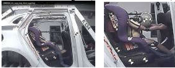
Figure 12a. Forward facing seat, initial position (left) and maximum forward excursion (right). (Jakobsson et al., 2013)
