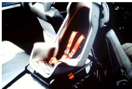
Fig 8b. Seat for front seat mounting from 1986 and rear seat mounting (with addition of support leg) 1990. (Photo: Volvo)
