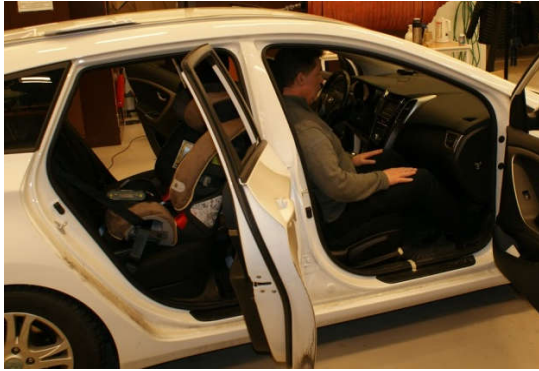
Fig. 14a. Adult sitting in front of a large rearward facing seat positioned in the rear seat. Britax Multitech in a Hyundai i30.
