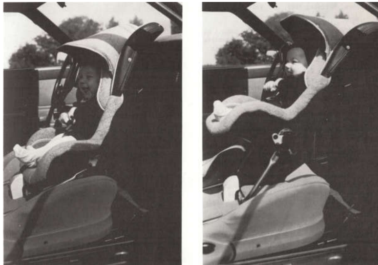
Fig. 6. Conventional rearward facing seat (left) with modification kit (right) that allows infants to travel in a reclined position (Turbell and Aldman, 1983)
