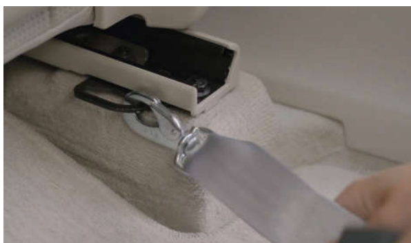
Fig 15a. Examples of pre-installed lower tether anchorages (Volvo XC90).
