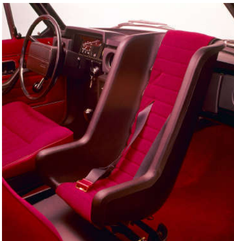
Fig. 4. Production seat by Volvo Sweden 1972, mounted on the seat chassis (left) or placed on top of front or rear seat (right). (Photos: Volvo)
