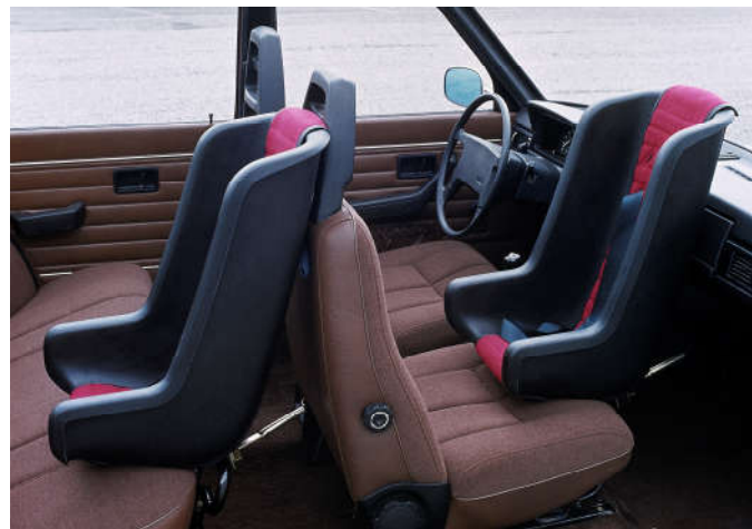
Fig. 4. Production seat by Volvo Sweden 1972, mounted on the seat chassis (left) or placed on top of front or rear seat (right). (Photos: Volvo)
