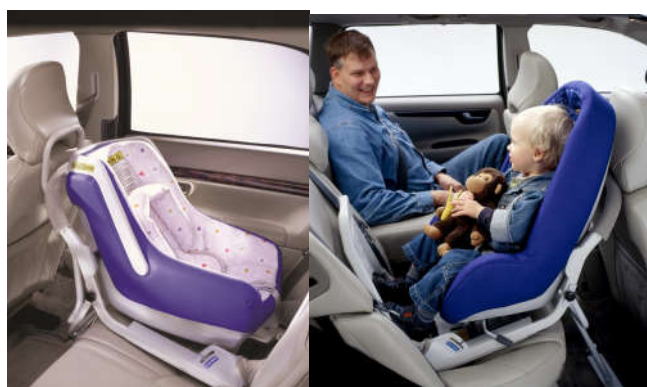
Fig. 9. World First rearward facing child seat with ISOFIX; Base with infant (left) or child seat (right). (Photos: Volvo)
