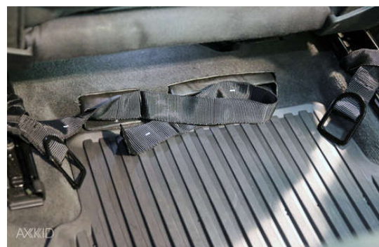
Fig 15b. Examples of lower tether anchorages; strapped around the seat rails.
