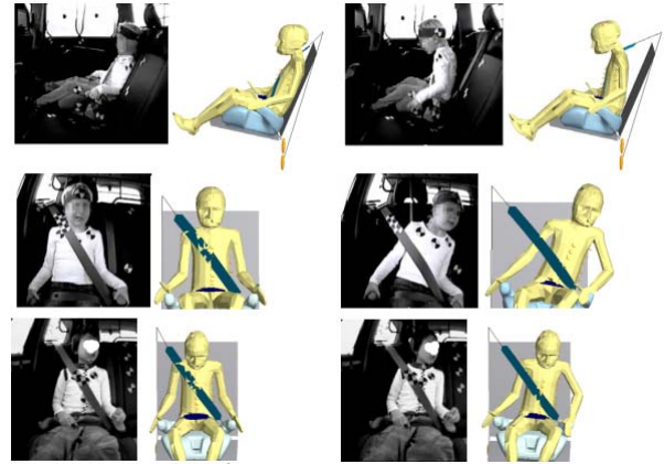
Figure 6. The active child HBM compared to volunteers at start and at maximum head displacement for a braking event (top row), a 0.8g steering event (middle row), and a 0.6g steering event (bottom row).
