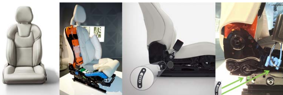
Fig. 2. Seat design of the WHIPS generation 2: overall seat design (left), seat-back structure (middle left), deformation elements (middle right and right).
