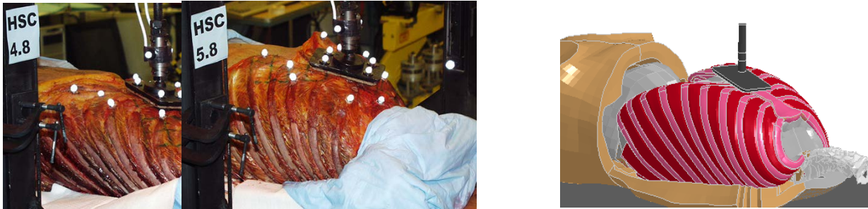
Fig. 1. Denuded thorax indenter impacts at mid-sternum (centre located at Rib 5). Left : pre-test 4.8 (adopted from Shaw et al. , 2007) [17]; middle : pre-test 5.8 (adopted from Shaw et al. , 2007) [17]; right : simulation model setup.
