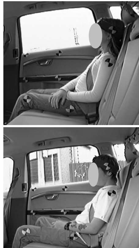
Fig. 6b. Examples of sagittal sitting postures 'aa' (top) and 'ab' (bottom) for children using seat belts only
