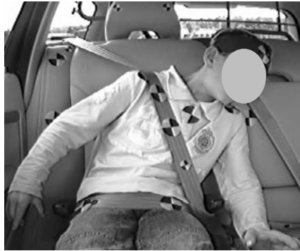
Fig. 9b. Example of leaning inboard for better visibility. Lateral sitting posture 'C+'.
