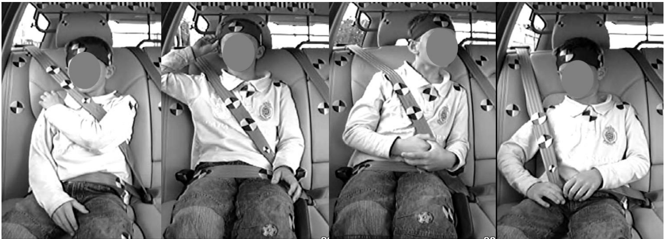
Fig. 4. Shoulder belt positions, from left to right: 'A', 'B', 'C' and 'D'.
