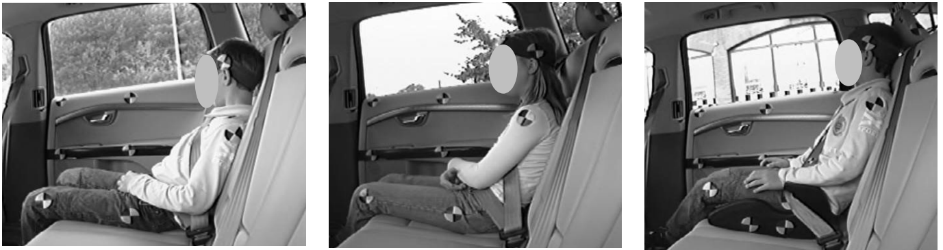
Fig. 7a-c. Examples of slouched sitting postures (left to right); a) sagittal sitting posture 'ea' seat belt restrained only, b) sagittal sitting posture 'eb' seat belt restrained only and c) sagittal sitting posture 'ea' when using booster.
