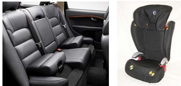
Fig. 1. The integrated Booster Cushion (IBC) and the high-back Booster (hbB) used in the tests.
