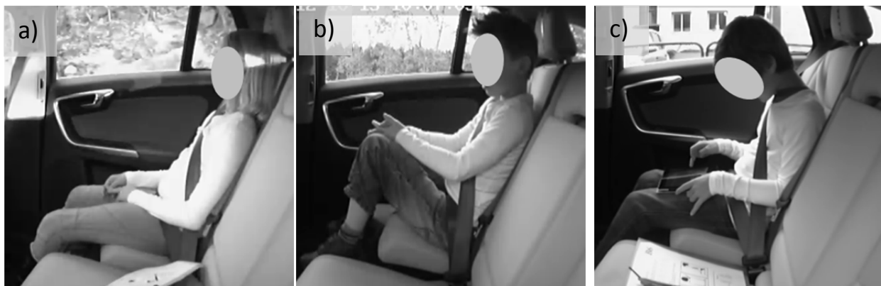
Fig. 4a-c. Examples of postures (left to right) with the entire back and shoulders against the seat back and head posture a) in contact with the seat back, b) upright, and c) leaning forward.
