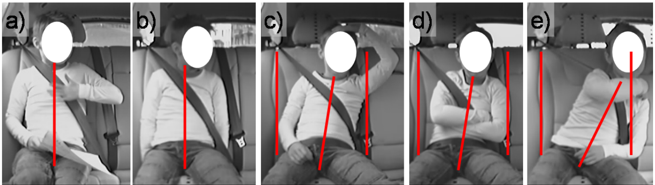
Fig. 2. Definitions of lateral sitting postures when seated on the IBC and shoulder belt positions a) upright posture and shoulder belt against the neck b) upright posture and shoulder belt on the mid-shoulder c) slight tilting posture and shoulder belt on the edge of the shoulder d) slight tilting posture and shoulder belt off the shoulder e) substantial tilting.
