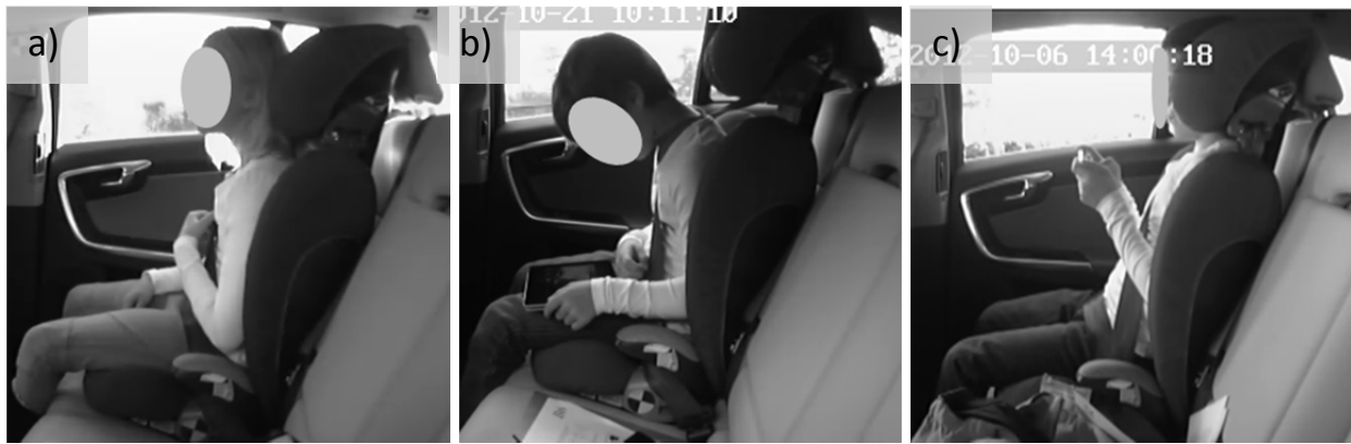
Fig. 5a-c. Examples of postures (left to right) with the entire back but not the shoulders in contact with the backrest and a) head posture upright, b) head posture leaning forward, and c) slouched torso posture and head posture in contact with backrest.
