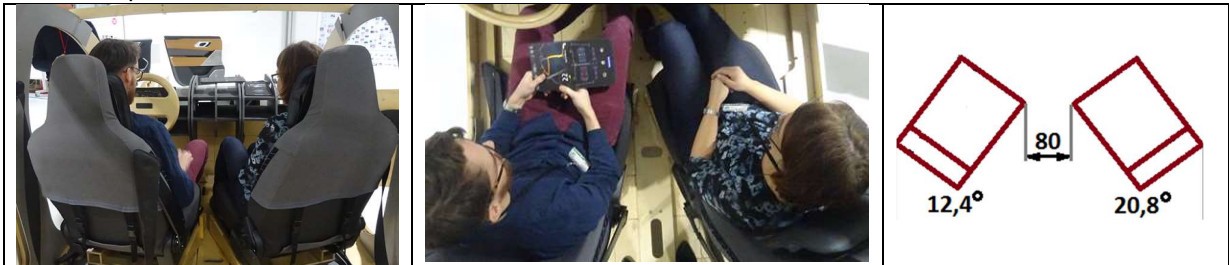
Figure 3 Rear view and top view of the seat configuration with 17^\circ inboard rotated front seats.
