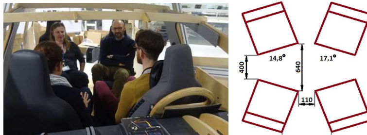
Figure 9 Face to face configuration, with all four seats rotated inboards 16^\circ .
