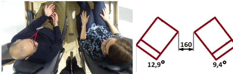
Figure 4 Top view of the seat configuration with 11^\circ inboard rotated front seats.
