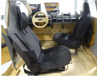
Figure 6 Two vehicle seats facing the direction of travel sideways.
