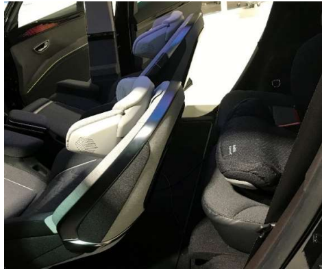
Figure 17 Example of reclined front passenger seat, reducing the space for the rear seat with a booster seat.
