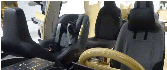
Figure 12 Incorrect installation of rearward-facing child seat in front passenger seat rotated 180° rearward facing.
