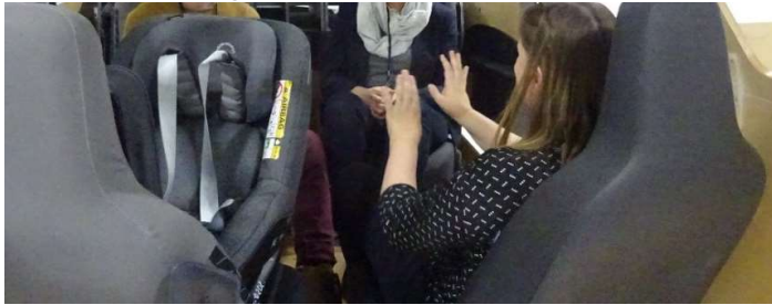
Figure 10 Installation of a child seat in a campfire position with 16° inboard rotation.
