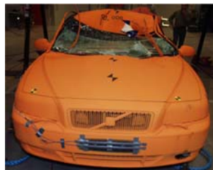
Fig. 13a. Photos of platform 1 vehicle after test at 70 km/h.
