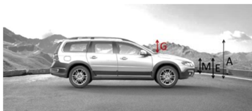
Fig. 3. Vertical deformation coding according to CDC, SAE J224.
