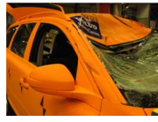
Fig. 13b. Photo of platform 2 vehicle after test at 70 km/h.
