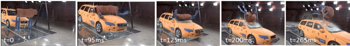
Fig. 11. Dynamic sequence of large animal dummy interaction with passenger vehicle, platform 2 vehicle test.
