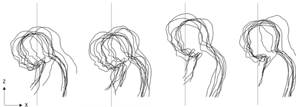
Fig. 6. Lateral silhouettes at maximum forward displacement for Shorter BC, Shorter IBC, Taller BC, and Taller IBC compared to common vertical reference line in the vehicle reference system. Plotted in the X (longitudinal) and Z (vertical) plane.
