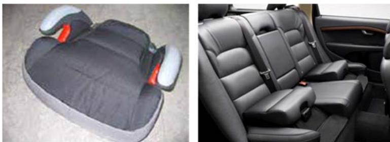
Fig. 1. Accessory booster cushion (left) and standard Volvo XC70 integrated booster cushion (right).
