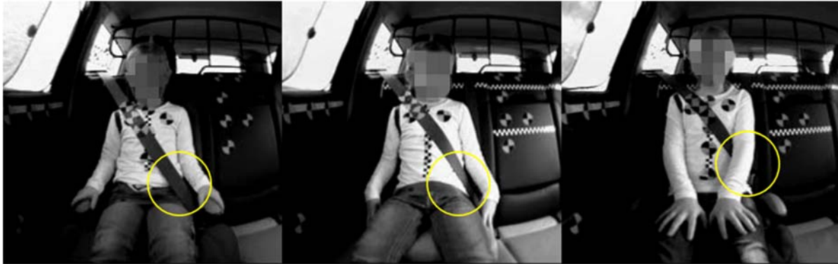
Fig. 2. Shoulder belt position on torso: (left to right) low, mid, and high.
