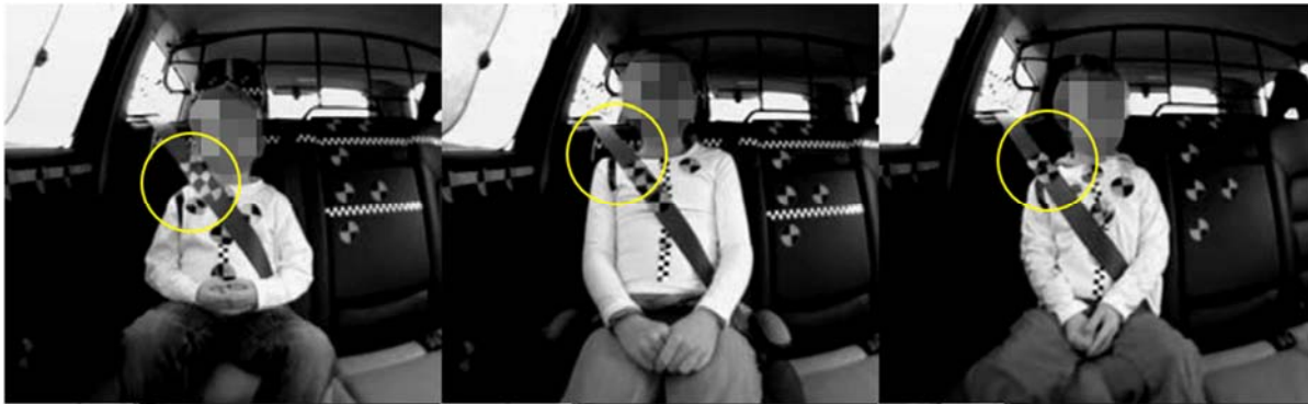
Fig. 4. Shoulder belt position on shoulder: (left to right) close to neck, mid-shoulder, and far out.
