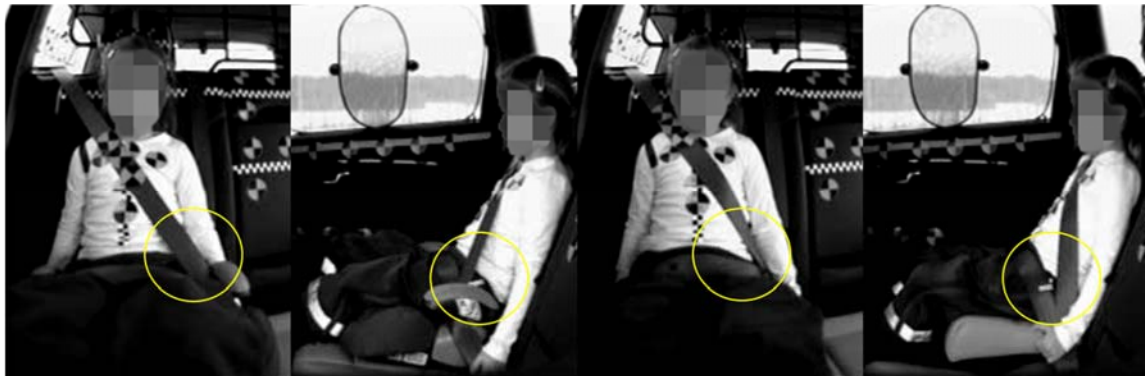
Fig. 3. Comparison of front and lateral views for an exemplar shorter child on the BC with gap (left) and on the IBC (right) without gap.
