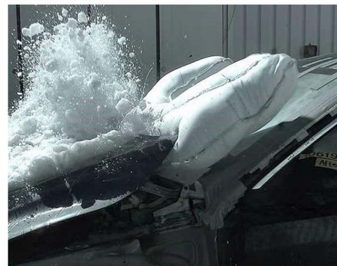
Figure 8. Activation test in a car packed with snow in the area of the pedestrian airbag module.
