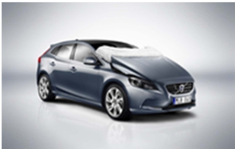
Figure 1. Deployed Pedestrian Airbag Technology in a Volvo V40.
