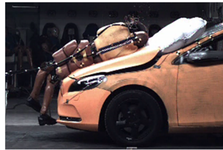
Figure 16. Full vehicle testing at speed 40 km/h impacting a 50%-ile male size prototype pedestrian dummy standing sidewise.
