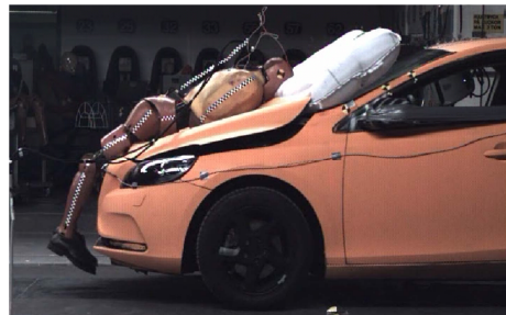
Figure 17. Full vehicle testing at speed 40 km/h impacting a 50%-ile male size prototype pedestrian dummy facing the vehicle.
