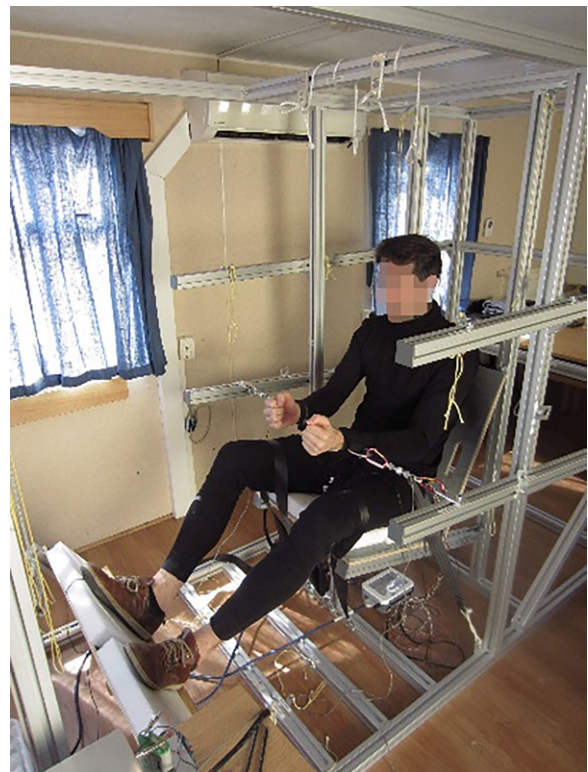
Figure 2. MVC test rig with volunteer.
