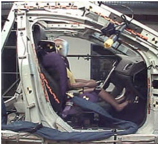
Fig. 2. Sled test set-up.
