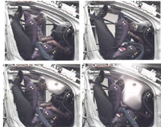
Fig. 8. Situation 11, Q6 forward leaning, forward seat position, pulse B; top row : tests without airbag; bottom row : with airbag. First airbag contact ( left ), max. forward position ( right ).
