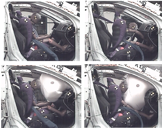
Fig. 7. Situation 12, Q6 forward leaning, mid-mid seat position, pulse B; top row : tests without airbag; bottom row : with airbag. First airbag contact ( left ), max. forward position ( right ).
