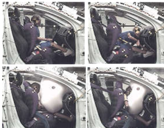
Fig. 9. Situation 15, HIII6y /Q6, belt placed under the arm mid-mid, seat position, pulse A; top row : tests without airbag; bottom row : with airbag. First airbag contact ( left ), max. forward position ( right ).
