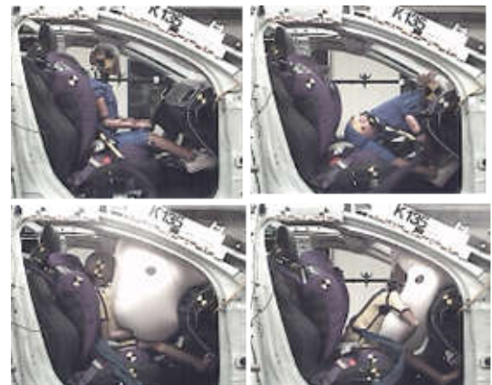
Fig. 10. Situations 16, HIII6y/Q6, belt placed behind the back mid-mid seat position, pulse A; top row : tests without airbag; bottom row : with airbag. First airbag contact ( left ), max. forward position ( right ).
