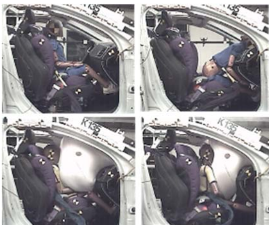
Fig. 16(c). Situation 14, HIII6y/Q6, belt placed behind the back , front-mid seat position, pulse A; top row : tests without airbag; bottom row : with airbag. First airbag contact ( left ), max. forward position ( right ).
