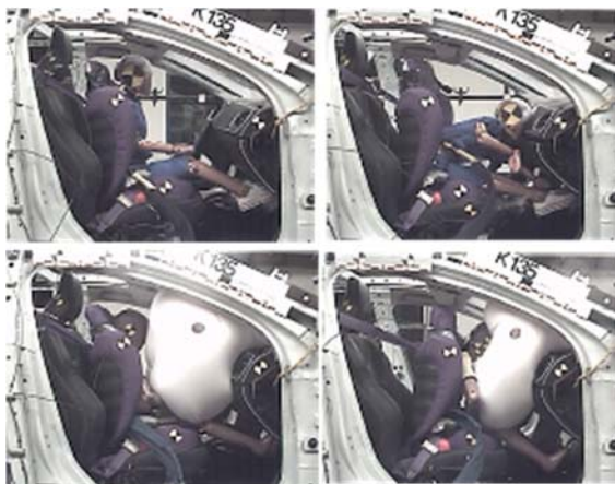
Fig. 16(a). Situation 15, HIII6y/Q6, belt placed under the arm mid-mid, seat position, pulse A; top row : tests without airbag; bottom row : with airbag. First airbag contact ( left ), max. forward position ( right ).
