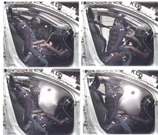
Fig. 12(b). Situation 13, Q6 forward leaning, mid-mid seat position, pulse A; top row : tests without airbag; bottom row : with airbag. First airbag contact ( left ), max. forward position ( right ).
