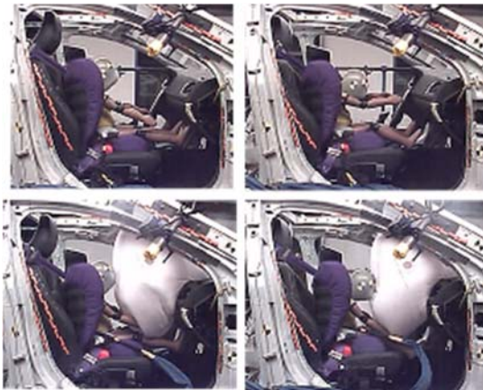
Fig. 10(a). Situation 3, Q3, mid-mid seat position, crash pulse C; top row : tests without airbag; bottom row : with airbag. First airbag contact ( left ), max. excursion ( right ).
