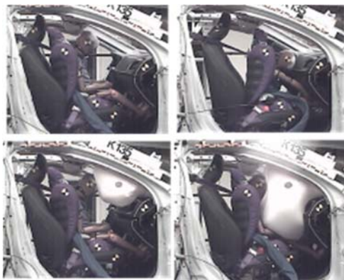
Fig. 14. Situation 11, Q6 forward leaning, forward seat position, pulse B; top row : tests without airbag; bottom row : with airbag. First airbag contact ( left ), max. forward position ( right ).
