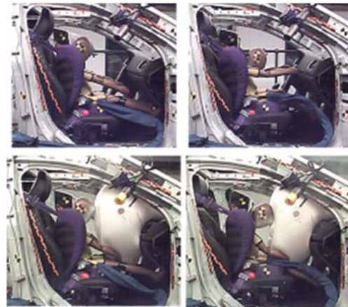
Fig. 10(b). Situation 7, Q6, mid-mid seat position, crash pulse C; top row : tests without airbag; bottom row : with airbag. First airbag contact ( left ), max. excursion ( right ).
