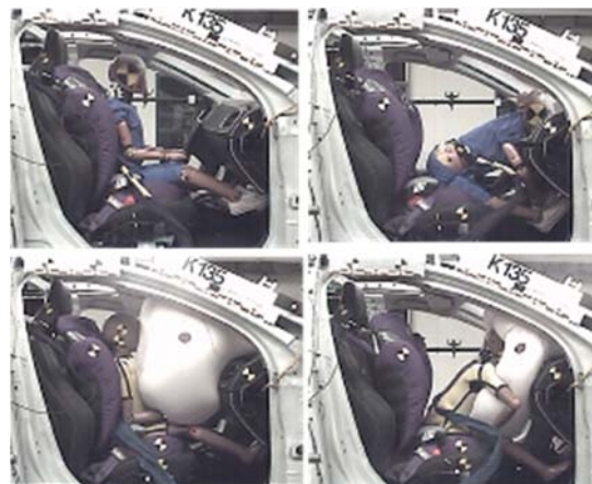
Fig. 16(b). Situations 16, HIII6y/Q6, belt placed behind the back mid-mid seat position, pulse A; top row : tests without airbag; bottom row : with airbag. First airbag contact ( left ), max. forward position ( right ).
