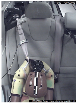
Q10update: Diagonal belt above inboard guiding loop of booster cushion
