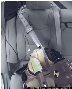
Q10update: Diagonal belt above inboard guiding loop of booster cushion
