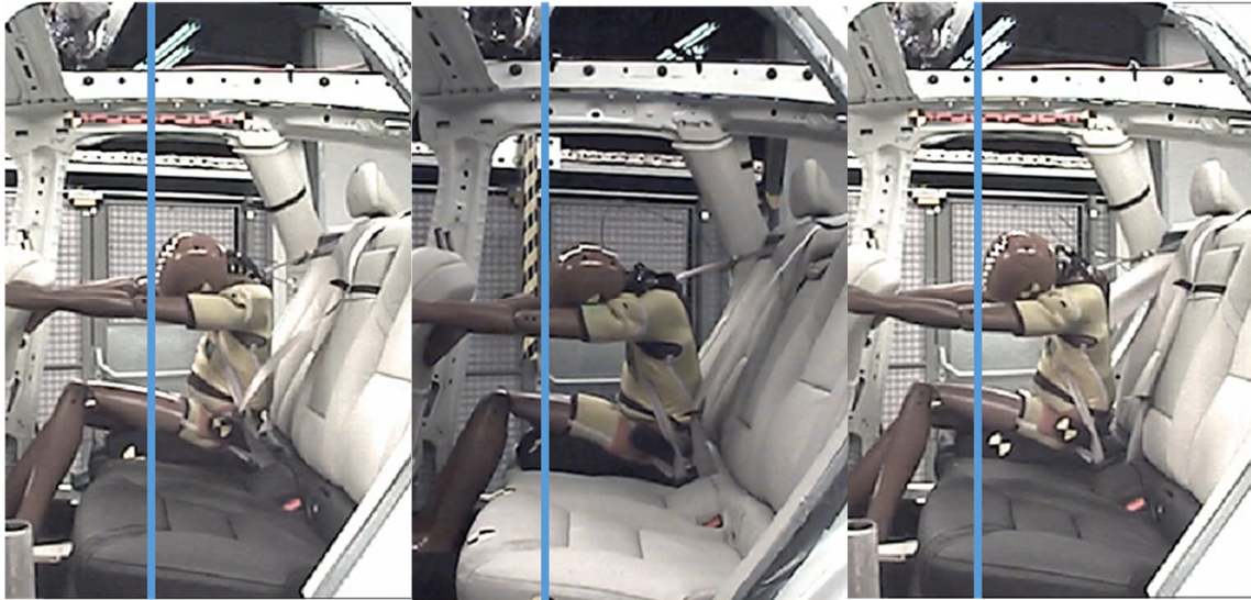
Figure 7. The kinematics of the Q10original (left), Q10update (mid) and Q10light (right) in ODB test at the time of max head excursion (vertical line).
