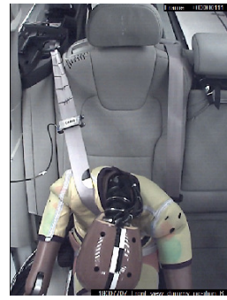
Q10update: Diagonal belt under inboard guiding loop, and dummy/booster cushion moved 15mm inboard
