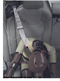
Q10original: Diagonal belt under inboard guiding loop, and dummy/booster cushion moved 15mm inboard
