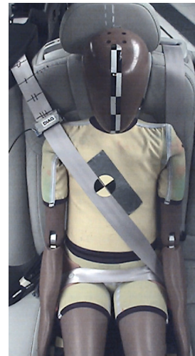
Diagonal belt under inboard guiding loop, and dummy/booster cushion moved 15mm inboard
