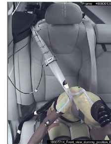
Q10update: Diagonal belt under inboard guiding loop, and dummy/booster cushion moved 15mm inboard
