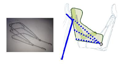
Figure 7a. Schematic restraint principles of straps around the child seat.
