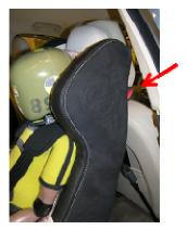
Figure 7c. Strap positioned around the front seat head restraint to secure support against the front seat.
