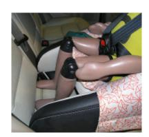
Figure 5c. The leg space area for a Q3 dummy in the CCS.
