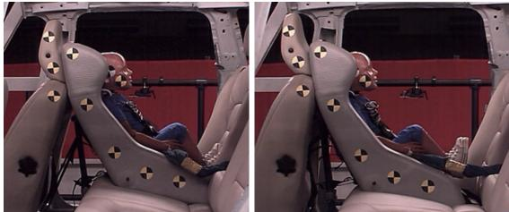
Figure 8a. Frontal impact, initial position. N.B. The seat is an early prototype with slightly different shape. The support leg is not in use in this test.
