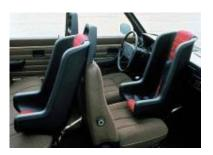
Figure 1a. The first child seat prototype (child harness removed) by Prof. Bertil Aldman in 1964 (Aldman, 1964). Crash tested in a Volvo PV444.
