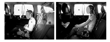
Figure 4. Forward excursion during braking for a shorter child to the left and a taller child to the right when seated on booster.
