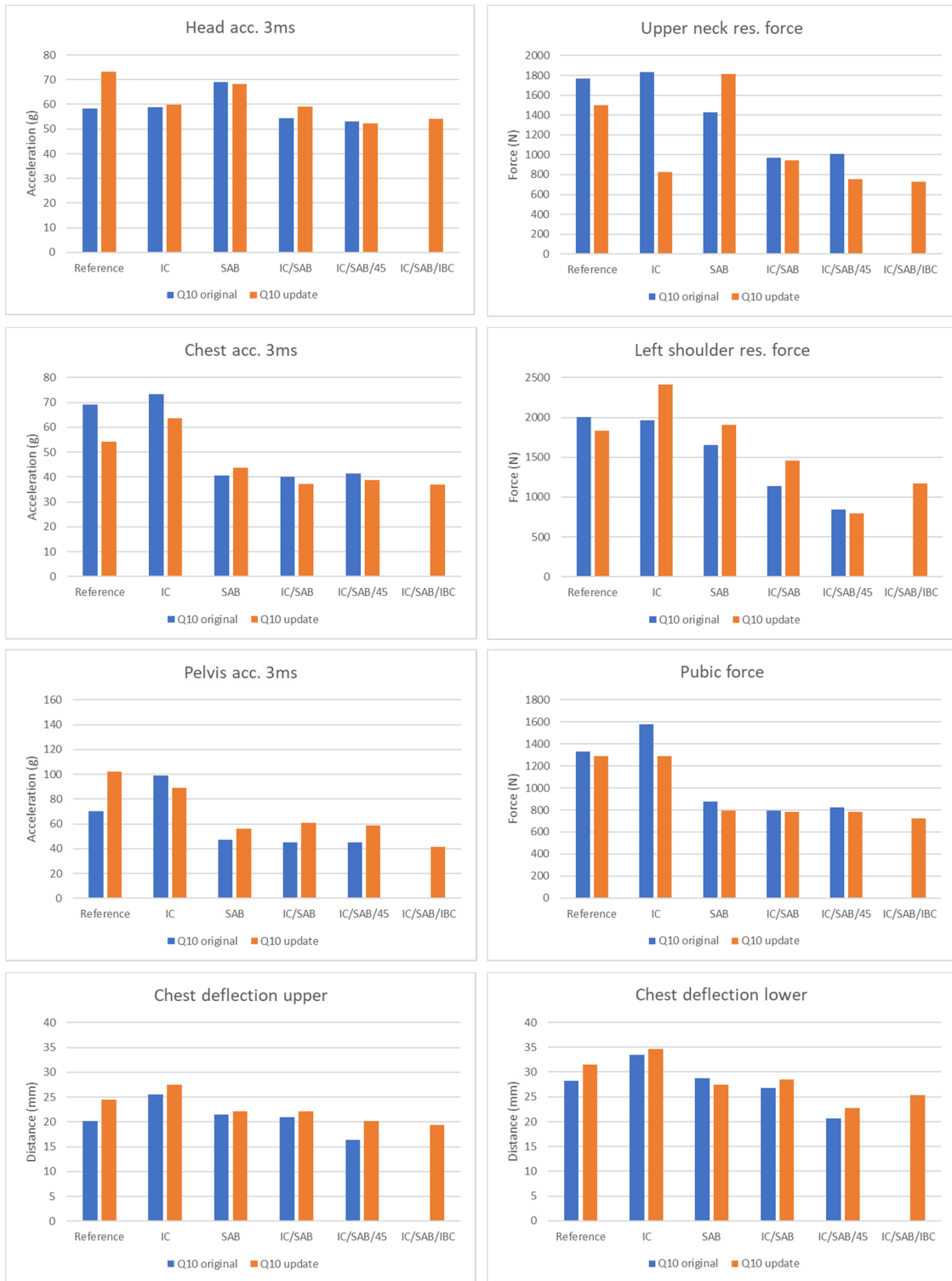
Figure 10. Head, neck, chest, shoulder and pelvis maximum responses for the Q10original and Q10update in the side impact tests.
