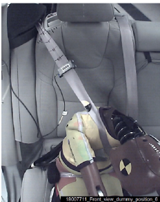
Q10update: Diagonal belt above inboard guiding loop
