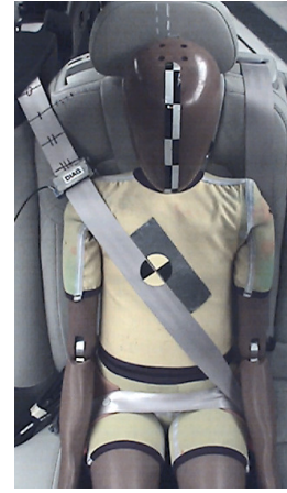
Diagonal belt under inboard guiding loop, and dummy/booster cushion moved 15mm inboard
