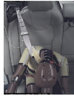
Q10original: Diagonal belt under inboard guiding loop, BC moved 15mm inboard
