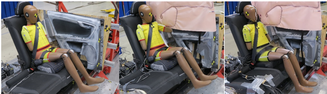
Figure 4. Side impact test set-up, Reference test (Q10original left), IC/SAB/45 test (Q10original mid) and IC/SAB/IBC (Q10update right).
