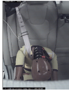
Q10original: Diagonal belt under inboard guiding loop
