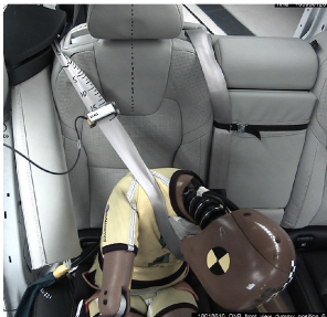
Q10light: Diagonal belt above inboard guiding loop
