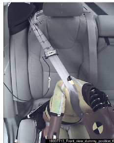
Q10update: Diagonal belt under inboard guiding loop
