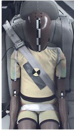
Diagonal belt above inboard guiding loop of booster cushion
