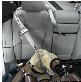
Q10light: Diagonal belt under inboard guiding loop
