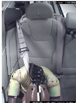
Q10update: Diagonal belt under inboard guiding loop
