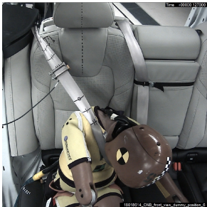
Q10original: Diagonal belt above inboard guiding loop
