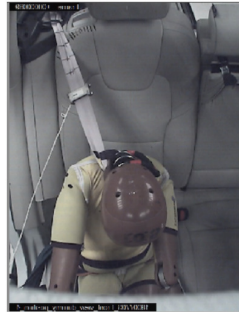
Q10original: Diagonal belt above inboard guiding loop
