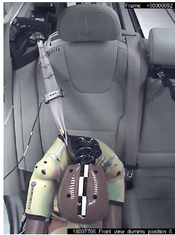
Q10update: Diagonal belt above inboard guiding loop
