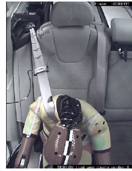
Q10update: Diagonal belt under inboard guiding loop, BC moved 15mm inboard
