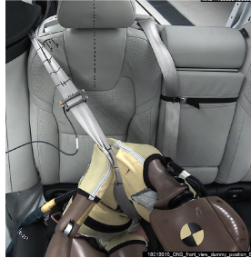
Q10original: Diagonal belt under inboard guiding loop
