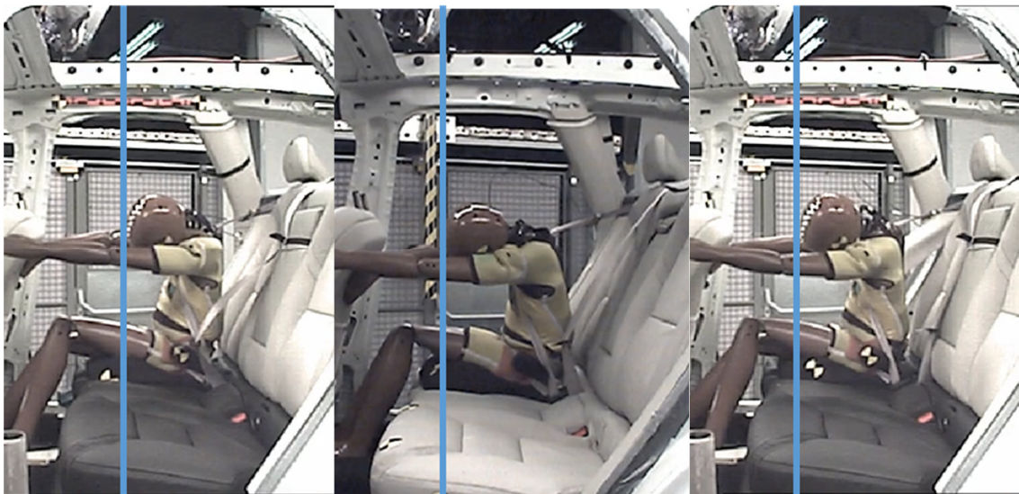
Figure 7. The kinematics of the Q10original (left), the Q10update (mid) and the Q10light (right) in the ODB test at time of maximum head excursion (vertical line).
