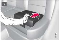
Figure 7a. Folding function from folded down adult seat position to low position.
