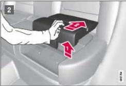
Figure 7b. Folding function from low to high position.
