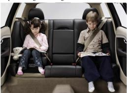
Figure 6. Photo of two children using the 2-stage integrated boosters.
