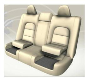
Figure 1. The new integrated 2-stage booster cushion, low and high position, respectively
