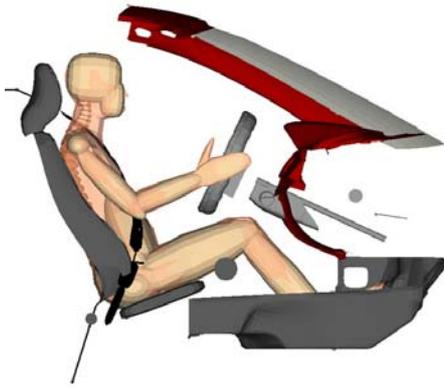
Figure 12a - Mathematical occupant model, in normal sitting posture, used in the parameter study of frontal impact (V).
