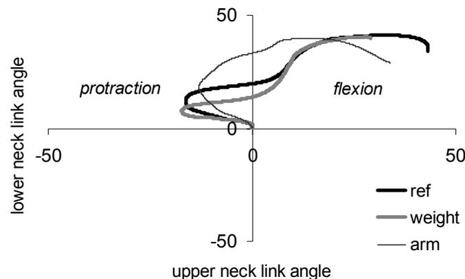
Figure 20 - Example of neck kinematics with upper neck link angle plotted versus lower neck link angle. Each quadrant represents a neck kinematics; upper left quadrant is protraction motion, upper right quadrant is flexion motion.
