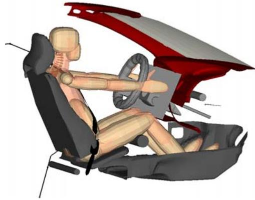
Figure 12b - Mathematical occupant model with simulated arm resistance to steering wheel in normal sitting posture.
