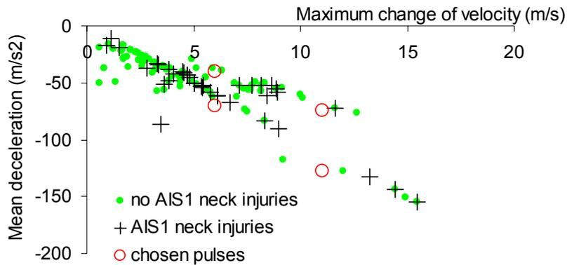
Figure 13 - Maximum change of velocity (max.  $\Delta v$ ) and mean deceleration of the chosen pulses in study (V) and the pulses in study (IV) including AIS1 neck injury information for the occupants.
