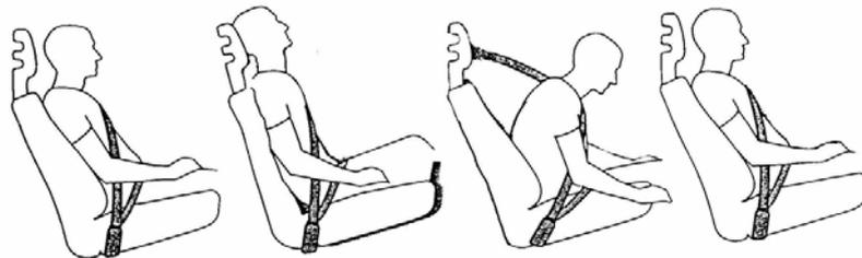
Figure 5 – General occupant motion in a rear-end impact.
