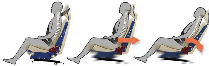
Figure 6 – WHIPS seat backrest motion in a rear-end impact
