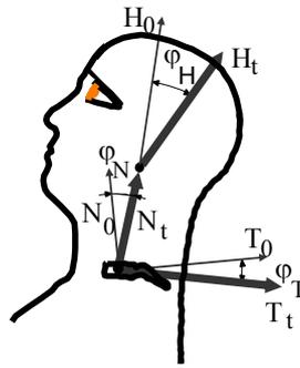
Figure 14 – Neck link model in 2D. The lines represent angular position at impact start 0 and at time t for T=T1 vertebra, N=neck link and H=head.
