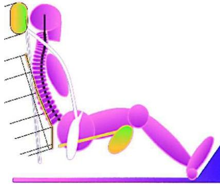
Figure 9 - Mathematical rear-end occupant model in MADYMO 2D. The lines perpendicular to the seat backrest and head restraint illustrate the borders of the different contact surfaces in the seat model.
