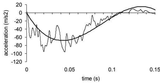
Figure 11a – An example of a DARR pulse including polynomial approximation of third degree.
