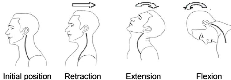
Figure 1 - General neck kinematics in a rear-end impact.
