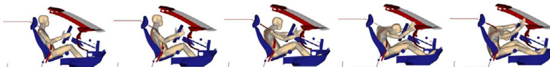
Figure 7 – General occupant motion in a frontal impact, no airbag deployment.
