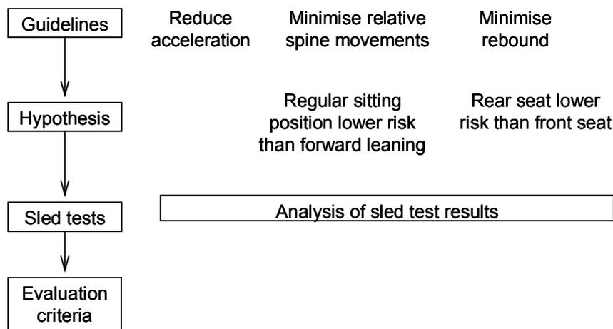
Figure 10 - Method in (II), describing the activities leading to evaluation criteria in rear-end impacts.
