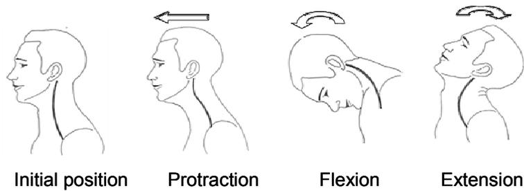
Figure 2 - General neck kinematics in a frontal impact.
