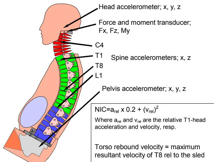
Figure 17. The BioRID I and instrumentation.
