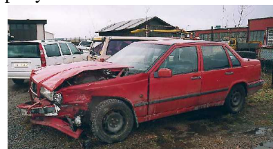
Fig. 5b - The Volvo 850 impacted by the car in case K1, K2, K3 and K5.
