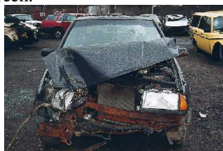
Fig. 3a - Photo of car in case N1, note the windscreen head indentation.
