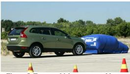
Figure 5. Target vehicle represented by an inflated balloon car.
