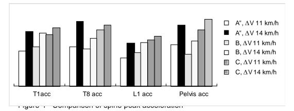
The body accelerations most closely related to the first guideline is suggested to be at the locations closest to seat interaction. As evaluation criteria for mapping occupant acceleration, the maximum of pelvis and spine L1 to T1 accelerations is suggested as evaluation criteria for this guideline.
