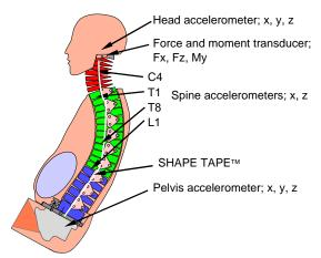
Figure 3 - The BioRID I and instrumentation
