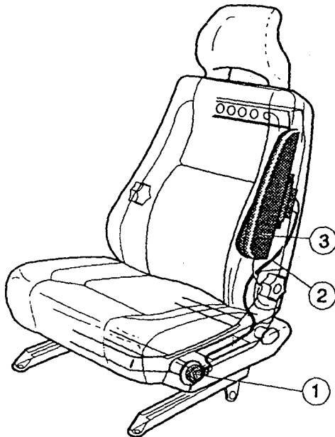
Figure 9. The Sipsbag system has sensor (1), non-el connection (2), and bag module (3) in the seat.
